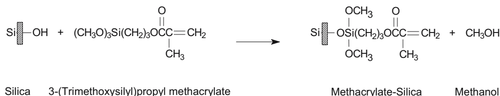
Fig. 1 Schematic representation of a silanization reaction
