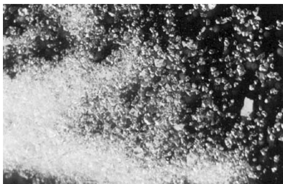
Fig. 3 Optical photomicrograph of silica (2 h) after disassociation (×18)
